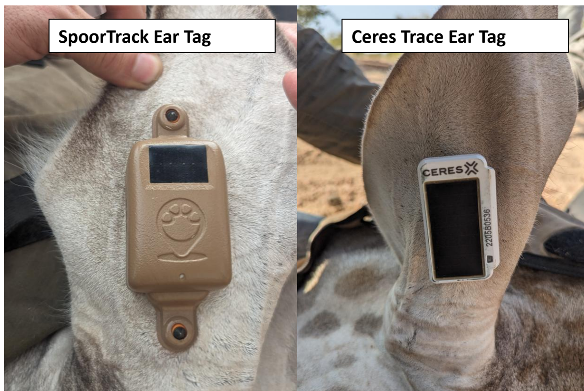
Figure 2: Examples of GPS tracking devices used on Nubian giraffe in the Boma Badingilo Jonglei Landscape.
