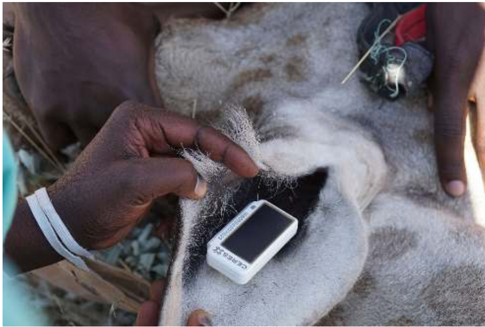
Figure 12: Ceres GPS ear tag fitted to the ventral (inside) of a southern giraffe ear. Image courtesy of GCF.
